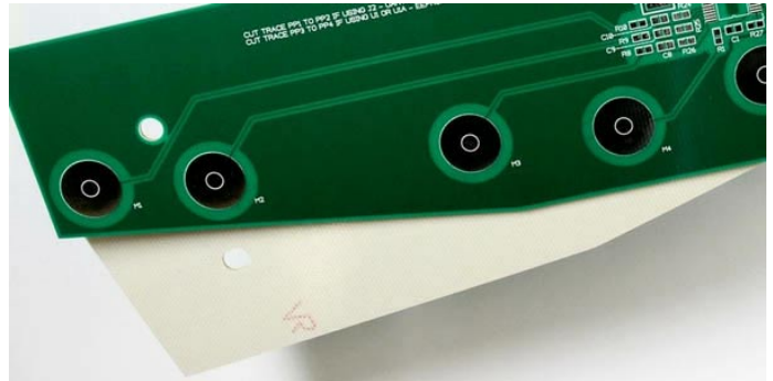
Fig. 1b - FR4 (2-sided epoxy-fiberglass)
