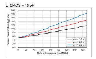
The actual current consumption is the total of the current under the condition of no load and the current to drive the output load (fo  $\times$  L\_CMOS  $\times$  V<sub>CC</sub>). To reduce the current consumption, it is effective to use lower frequency, lower supply voltage and lower output load.
