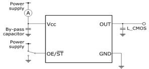
\* Disable current test should be OE = GND. Stand-by current test should be  $\overline{ST} = GND$ .
