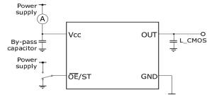
\* Disable current test should be  $\overline{OE} = \overline{V_{CC}}$ . Stand-by current test should be  $ST = V_{CC}$ .
