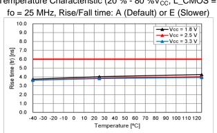
Temperature Characteristic (20 % - 80 %V<sub>CC</sub>, L\_CMOS = 15 pF)
