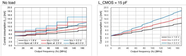
The actual current consumption is the total of the current under the condition of no load and the current to drive the output load (fo x L\_CMOS x V<sub>CC</sub>). To reduce the current consumption, it is effective to use lower frequency, lower supply voltage and lower output load.
